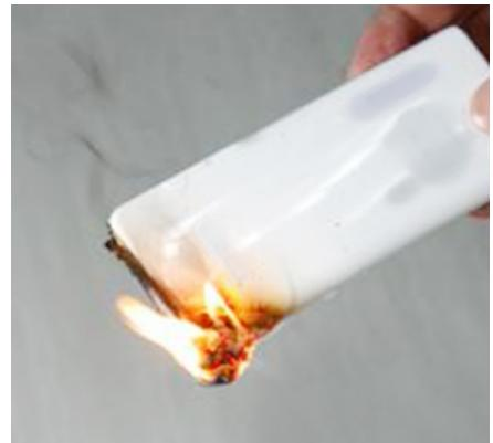
It is used to test flame retardant properties for the insulated enclosure of household appliances, switch panels, printed circuit boards, and insulating materials.
