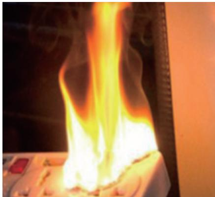
It is used for the test of ignition hazard of electronic and electrical products, the evaluation of hot burning performance and the test of high temperature resistance.
