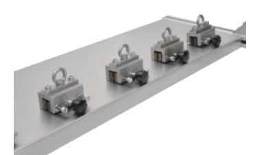
The tester can make six specimens at a time, and the tooth surface of the fixture adopts special anti-loose treatment, which is manually clamped, convenient and reliable.
