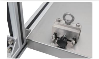
The fixtures and weights of the tester are designed in stainless steel for corrosion resistance and long service life.
