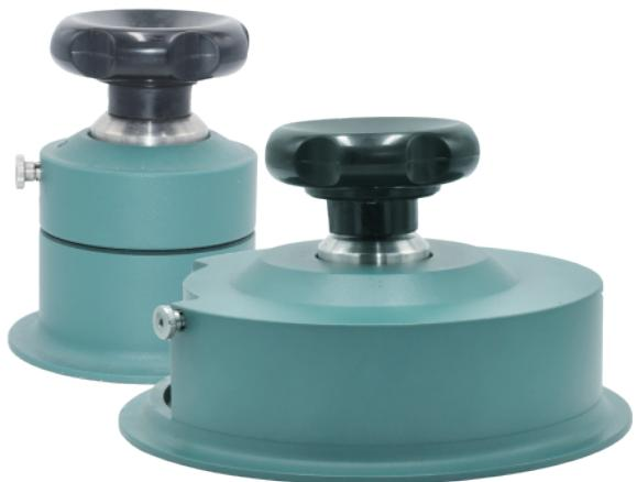
2.This instrument with an integral design mainly consists of outer cover 、 handle、 blade fixing rack and rotation table .
