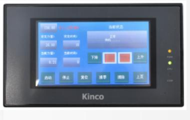
Microcomputer control system is more efficient and reliable, which can be used to program by 7-inch color LCD touch screen and achieve control, detection, calculation, data display and other functions.
