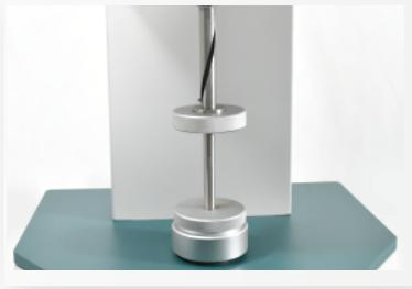
The tester adopts a stepping motor to drive the screw rod up and down to realize loading, precise control, stepless pressure, and the loading force can be corrected, which is with functions of zero clearing, convenient and high efficiency.
